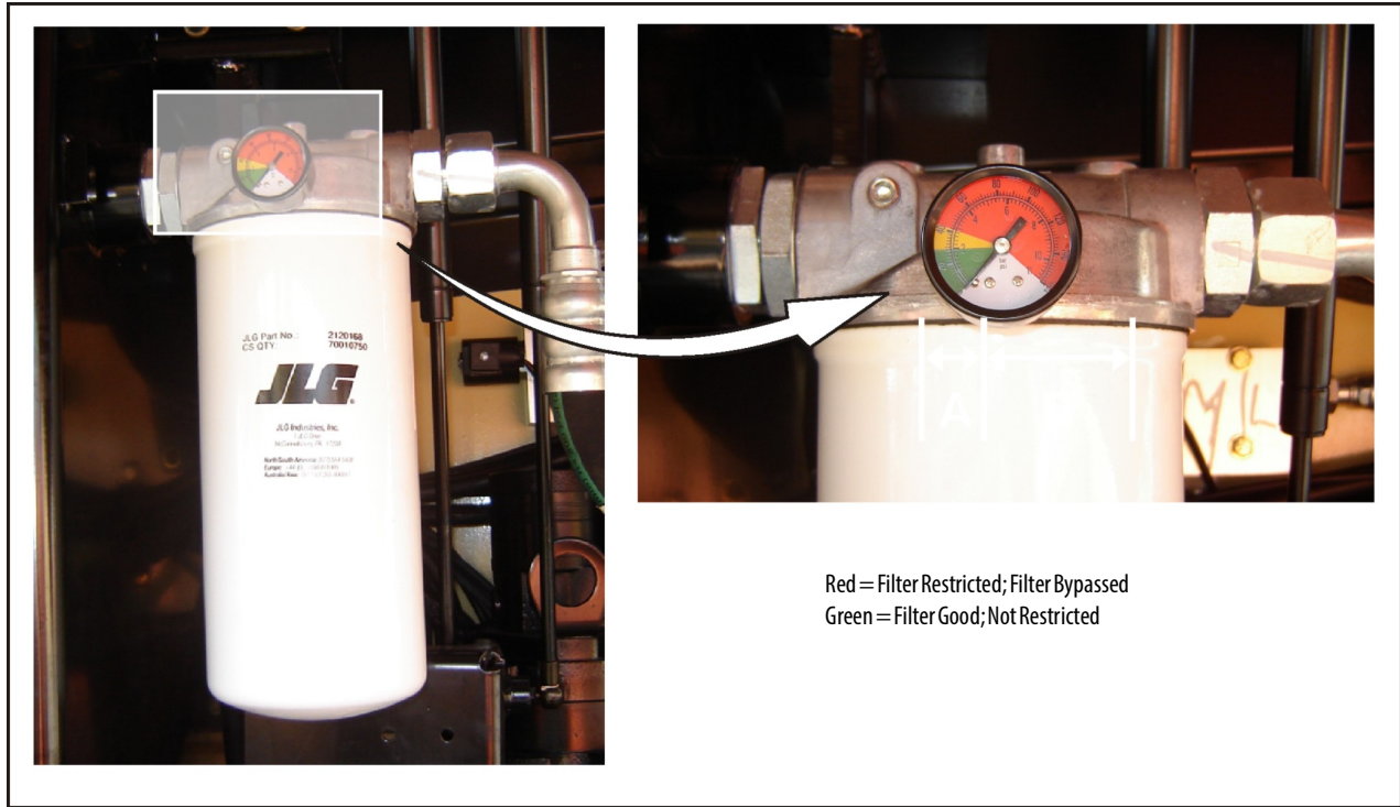
Figure 7-9. Hydraulic Return Filter Condition Indicator - S/N 139396 to Present
